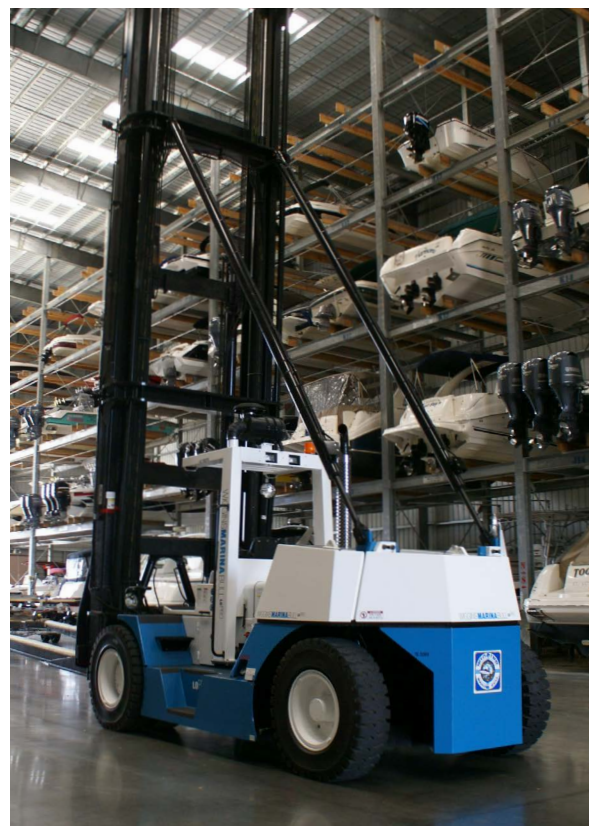
WIDE VIEW MAST The Wide View mast allows the operator an unobstructed center-line view.
